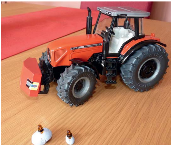
Rear wheel weights fitted, paint applied to the wheel hubs and cab lights, whilst the beacons are drying and awaiting fitting to the can top.
